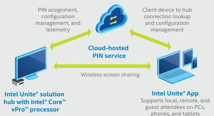
The **Intel Unite® Cloud Service option** connects directly to the Intel Unite® solution PC hub and supports the Intel Unite client app
